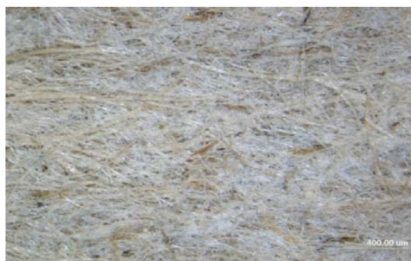
Figure 4.5 Aligned alkali treated fibre mat produced by dynamic sheet forming (DSF).
