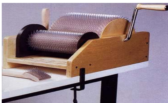
Figure 4.3 Hand carding machine used to produce aligned long fibre mats.
