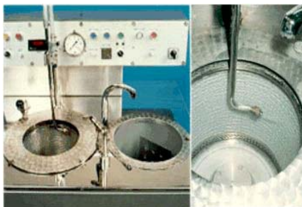
Figure 4.4 Dynamic sheet former used to produce aligned short fibre mats.
