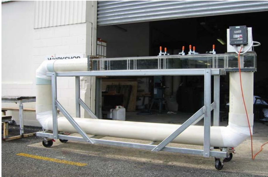
Figure 2.4. 2 metre, 230 litre recirculating flume.
