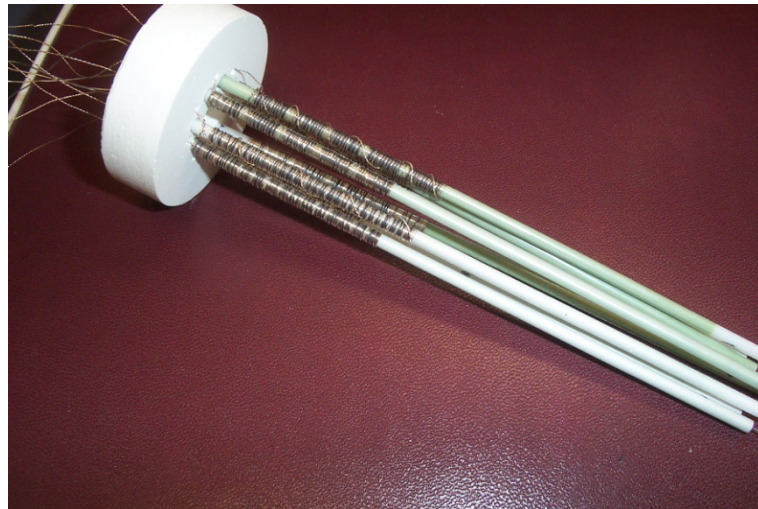
Figure 5-4 Alumina fibre manifolds (P7)
