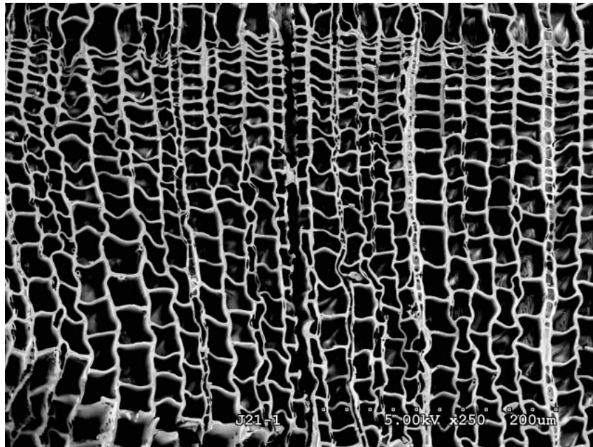
Figure 1.4: Micrograph of a transverse section of Picea sp. wood with brown rot showing the fungus has degraded some cells completely but not others. Cells have collapsed and have a “wavy” appearance (Source Joel Jurgens, unpublished micrograph).
