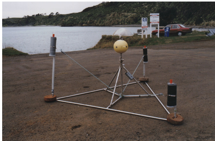
Figure 11: S4 current meter mounted on a frame ready for deployment in the surf zone.
