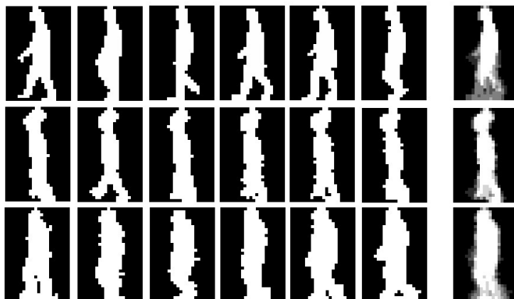
Figure 5.1: Extremely low quality gait sequences (derived from videos with frame-rate at 1 fps and resolution of 32 \times 22 pixels). Top/middle row: from the indoor OU-ISIR-D [Makihara et al., 2012] database with low/large gait fluctuations; bottom row: from the outdoor USF database [Sarkar et al., 2005]. In each row, the rightmost image is the AGI corresponding to the whole gait sequence.
