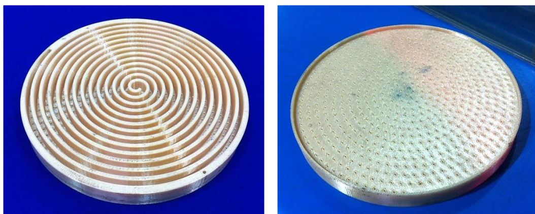
Figure 4.5 – Rapid prototype spiral distributor (a) Front, (b) Back
