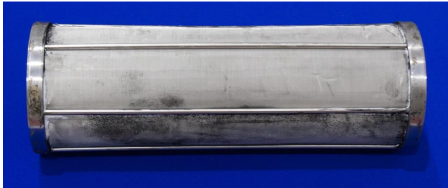
Figure 4.8 – Large generator filled with carbon and wrapped in glass filter and gauze
