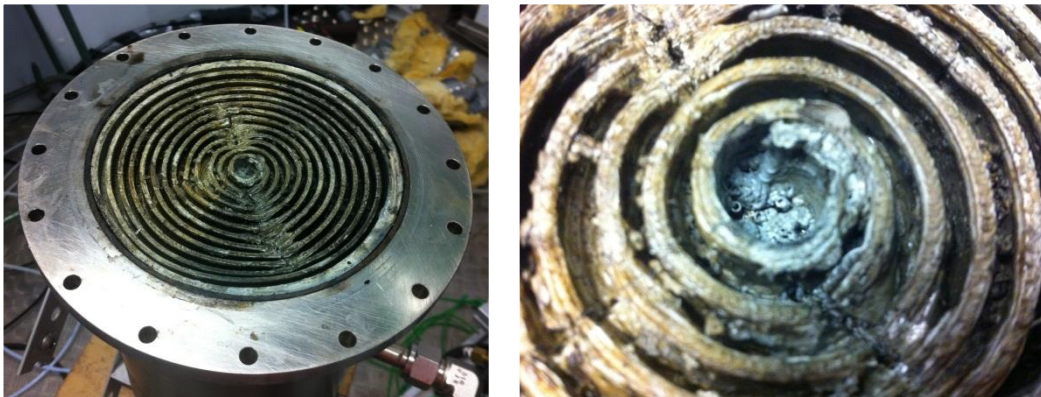
Figure 9.18 – (a, b) Damaged water distributors after testing
