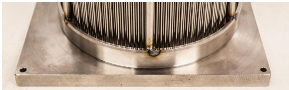
Figure 4.3 – End plate of large generator
