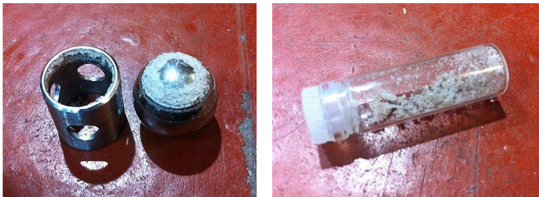
Figure 8.22 – (a) Salts adhered on check valve components, (b) Salt crystals found obstructing and blocking check valves
