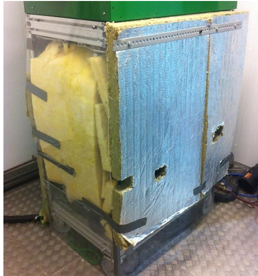
Figure 9.1 – Insulated heat pump during testing
