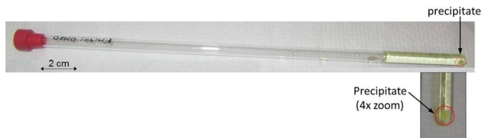
Figure 4.12 Precipitate from the photo-irradiation of complex 40 (4 mM) with DMPO (8 mM) with 463 nm light prepared in PBS/D 2 O at pH* 7.4. Magnified (4x) image of precipitate in the included inset.
