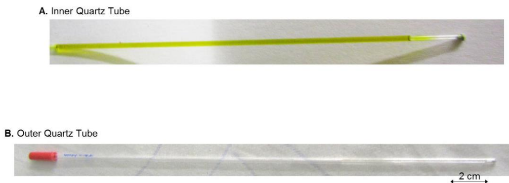
Figure 2.1 EPR tubes used in this work; (A) inner quartz EPR tubes with inset depicting the EPR tubes sealed with T-Blu Tac® at one end, and (B) larger 2.0 mm O.D outer quartz EPR tubes.
