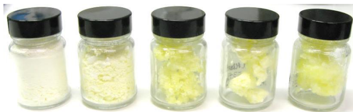
Figure 3.18: Image of PPDL- b -PEHA copolymers described in Table 3.4 (Left to right: DP PPDL:PEHA = 1:1, 1:2, 1:4, 1:7.5, and 1:13).
