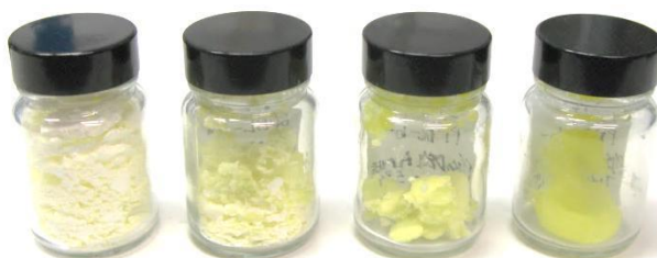
Figure 3.19: Image of PPDL- b -PIDA copolymers described in Table 3.5 (Left to right: DP PPDL:PIDA = 1:1, 1:2, 1:4.3, 1:6).
