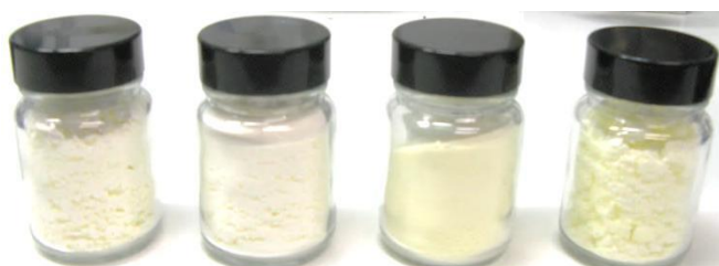
Figure 3.21: Image of PPDL- b -PSA copolymers described in Table 3.7 (Left to right: DP PPDL:PSA = 1:1, 1:2.5, 1:4, 1:10.6).
