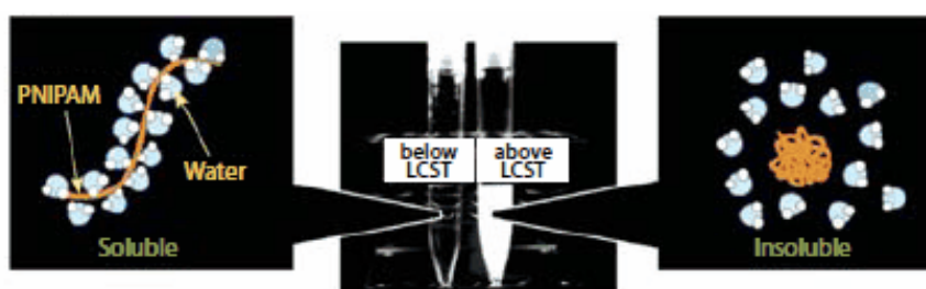
Figure 1.20: Images showing the ordering of the water molecules around the PNIPAM polymer below the LCST cloud point, resulting in a dissolved polymer, and the macroscopic precipitation that occurs upon heating above the LCST cloud point of the polymer 120
