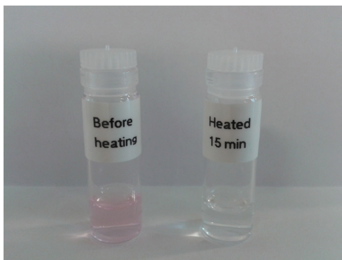
Figure 5.20: Left) encapsulated Nile Red in micelles of 4.02 Right) micelle solution after heating to unimers and removal of Nile Red by filtration
