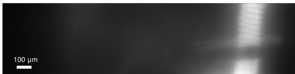
Figure 4.7: This image of the emission from an illuminated filament lamp among the first acquired using the completed XEOM optics and detector. 8 It is possible to distinguish the filament coils themselves and one of the filament support structures within the bulb (the dark shadow across the coils).
