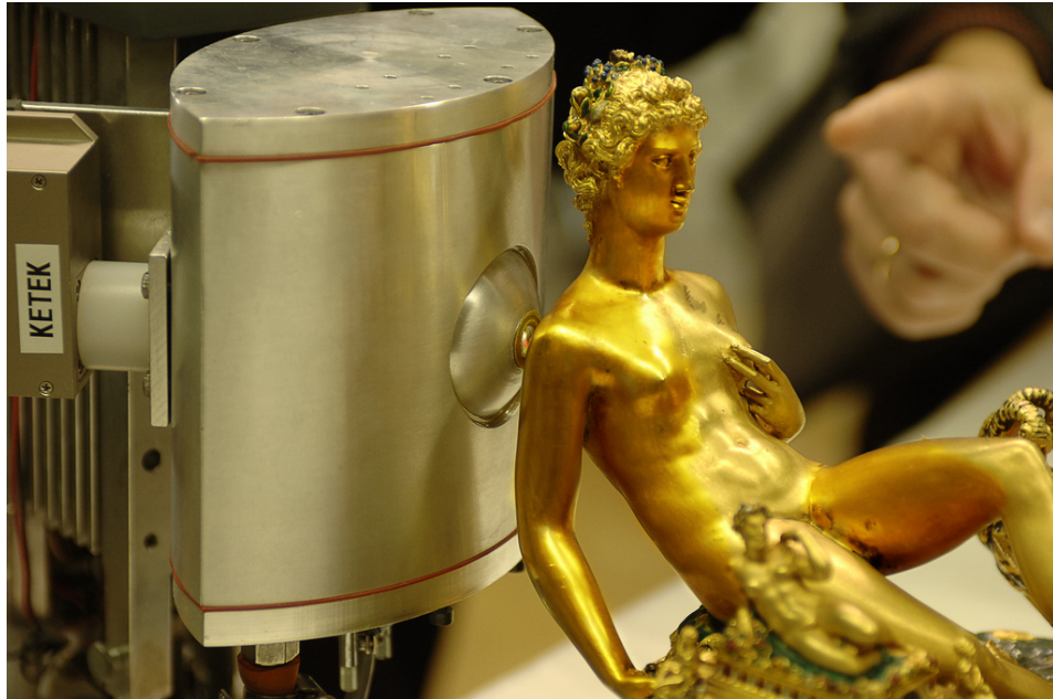
Figure 1.1: XRF analysis of a 16th-century salt cellar made of gold, ebony and enamel at the Kunsthistorische Museum, Vienna, Austria. Credit: Dean Calma / IAEA
