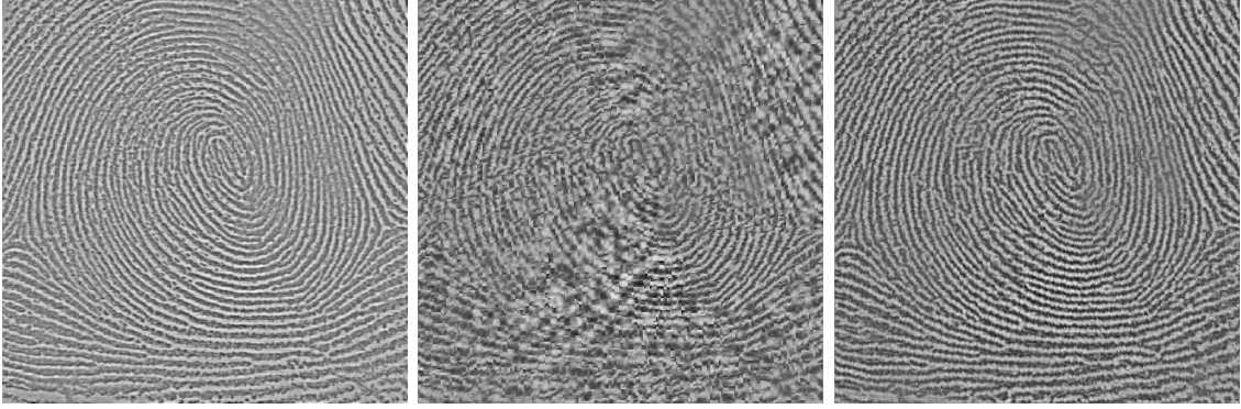
Figure 1.5: Finger print image test: (left)original image,(middle)reconstruction by two-component method, (right) by modified EM for GMM
