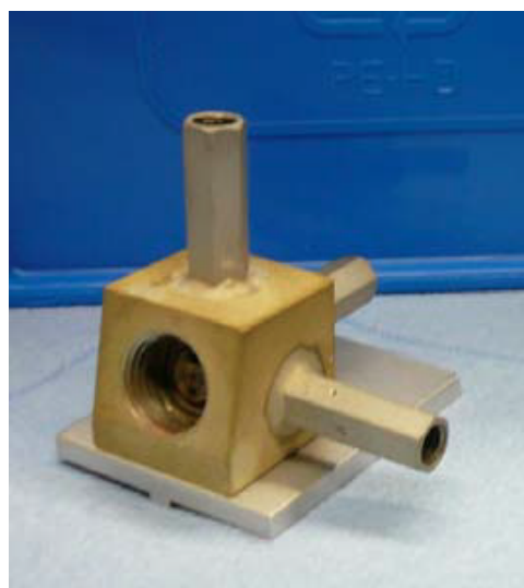
Figure 4.2 An example of an initial metallic (steel) coupling device built in the Max Plank Institute of Light, Erlangen used in the first PCF-MS system (Figure 4.3).
