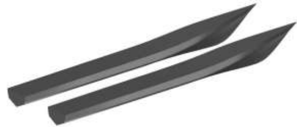
Figure 1. 3D model of high speed “deep-V” catamaran model.
