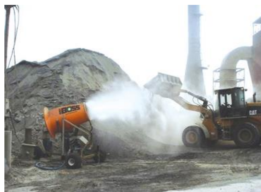
Figure 11. Dust boost at stock pile area
