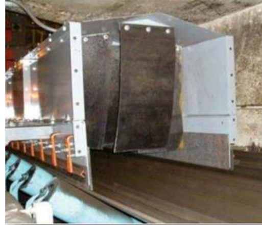
Figure 9. Rubber curtain inside the chute
