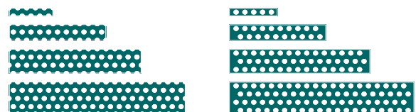
Fig. 10. Representation of beam samples of increasing size generated by finite element meshes shown in Figs. 9 (right) and 11 (left).
