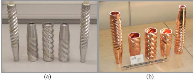
Fig. 4. (a) Machined aluminum formers. (b) Final copper waveguides.
