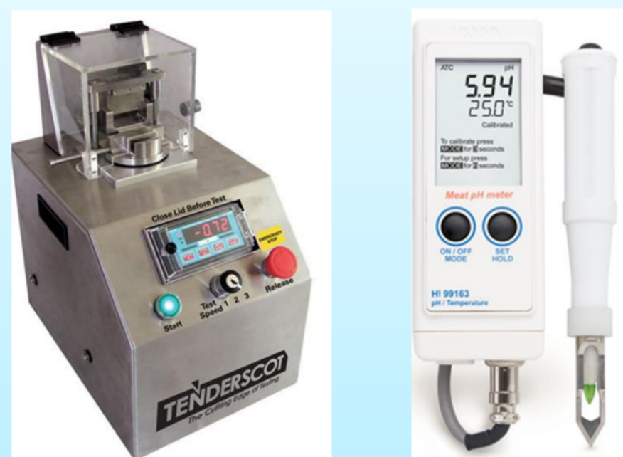
Fig.2. Instruments for measuring beef eating quality. (a) Meat tester (b) pH meter
