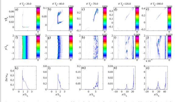
**Figure 4.** The phase space (1st row), two-dimensional density distribution (2nd row), and one-dimensional density distribution (3rd row) of protons, plotted by averaging over  $-0.5\lambda_{\rm L} < y < 0.5\lambda_{\rm L}$ , at times  $t = 20T_{\rm L}$ ,  $40T_{\rm L}$ ,  $70T_{\rm L}$ ,  $120T_{\rm L}$  and  $180T_{\rm L}$ .
