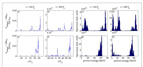
**Figure 7.** The one-dimensional density distributions (the first two columns) and energy spectra (the last two columns) of protons within  $|y| < \lambda_L$  at  $t = 150T_L$  and  $t = 300T_L$  between the original case of  $n_{e0 \text{ max}} = 10n_{cr}$  (the 1st row) and the case with doubled peak density  $n_{e0 \text{ max}} = 20n_{cr}$  (the 2nd row).
