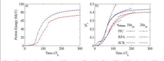
Figure 8. The evolutions of proton (a) energy and (b) momentum. Theoretical predictions of RPA and SCR are shown in panel (b).
