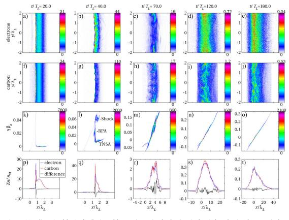
**Figure 2.** Two-dimensional density distributions of electrons (1st row) and carbon ions (2nd row), the carbon ion phase space (3rd row), and the one-dimensional density distribution (4th row) of electrons, carbon ions, and their differences, which are plotted by averaging over  $-0.5\lambda_{\rm L} < y < 0.5\lambda_{\rm L}$ , at times  $t = 20T_{\rm L}$ ,  $40T_{\rm L}$ ,  $70T_{\rm L}$ ,  $120T_{\rm L}$  and  $180T_{\rm L}$ .
