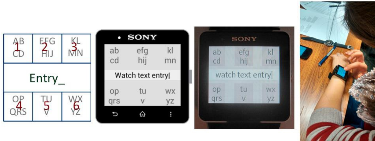
Figure 1: Evolution of our prototype implementation on a Sony SmartWatch 2 (from left: concept, design, implementation, use)
