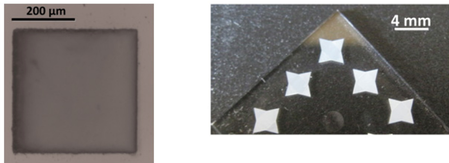
Fig. 12. Examples of crack-free micro-milling of fused silica with NCF-delivered ps pulses.
