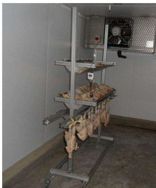
Figure 28. Trolley with perforated shelves and shackles used for chilling of partially (placed on shelves) and standard (placed on shackles) eviscerated poultry carcasses
