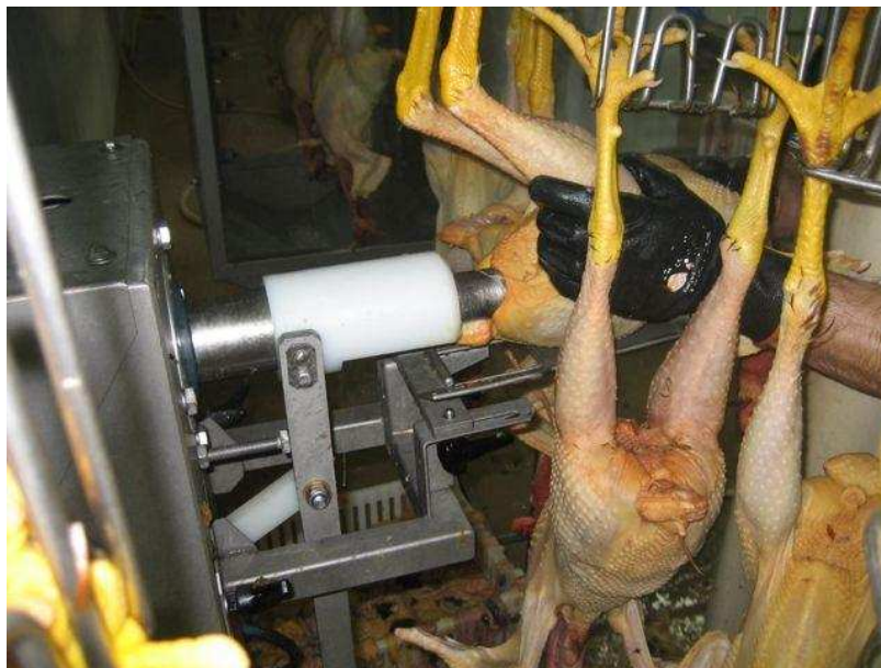
Figure 19. Bayle Annular Knife Vent Cutter machine with central vacuum
