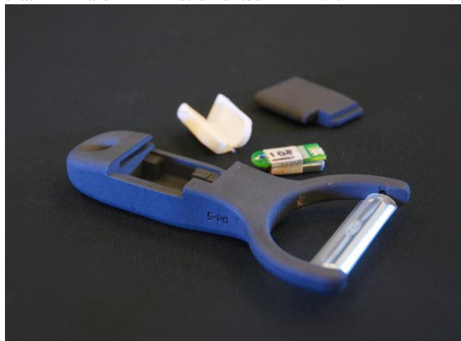
Figure 2. An off-the-shell peeler re-built to house a WAX (seen behind the peeler with its white casing)
