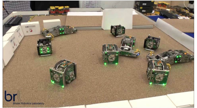
Figure 4: Swarm Phase: Robot performing collision avoidance and random walk.
