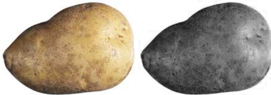
(a) Example white potato affected by (b) Clearer to the human eye in the blue black dot. colour channel.
