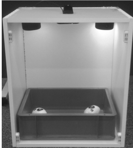
Figure 1. Image acquisition - A tray containing potatoes is placed inside the light box, then the box is closed by placing the door on the front (not shown in the picture), attached with magnetic fixings, and an image is captured from the overhead camera for analysis by the system.
