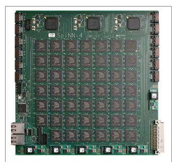
FIGURE 1 | A 48 chip SpiNNaker board (228  $\times$  233 mm), the building block from which larger systems will be constructed.
