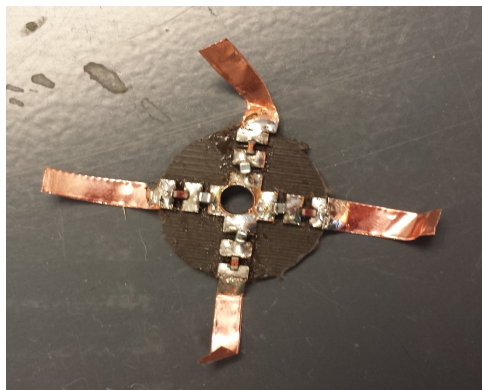
(c) Cooper tape to ensure electrical contact
