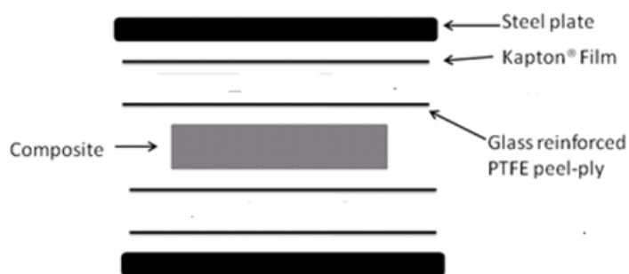
Figure 3.4: Schematic set up of laminate manufacture using hot press
