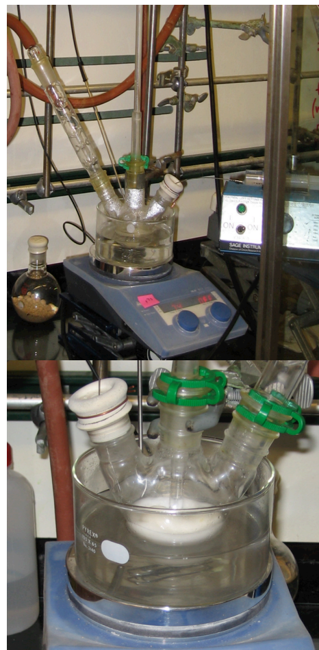
Figure 3.5: Typical set-up for HPG synthesis (top) and after all the glycidol has been added the HPG becomes very viscous (bottom).
