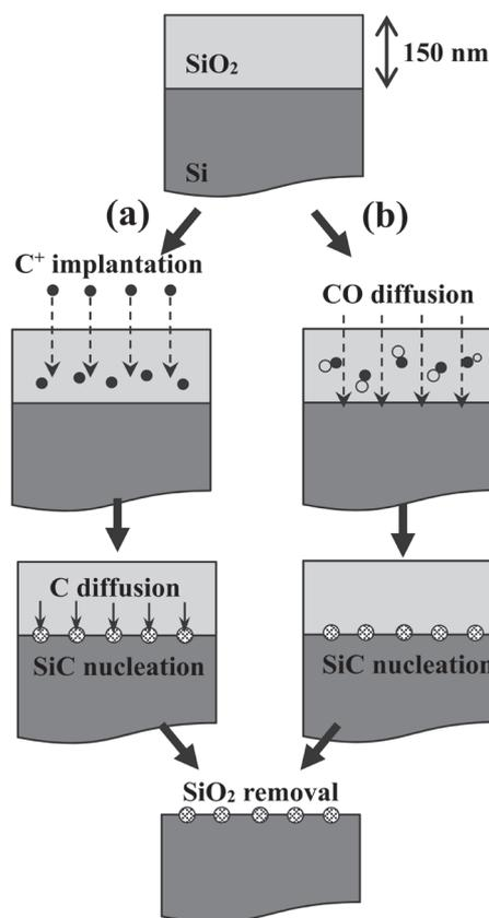
Fig. 1. Formation processes of SiC NCs in SiO<sub>2</sub>/Si samples by C ion implantation (a) and CO thermal diffusion methods (b).
