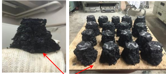
Specimens after the CS test
