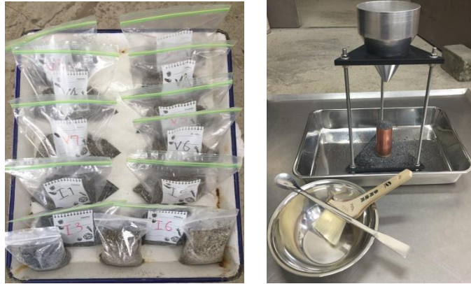
Figure 41. Test setup for assessing fine aggregate angularity
