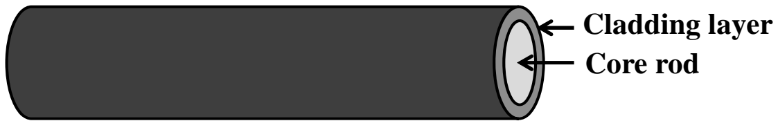
Figure 1-17: A clad cylindrical buffer rod
