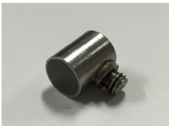
Figure 2-9: A longitudinal ultrasonic transducer with operating frequency of 5MHz
