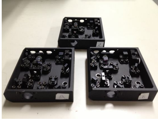
(c) Three optical sensors for spindle motion measurement
