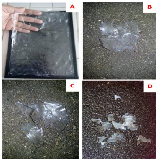
Figure 7. Biodegradable plastic decomposes in soil (a) 0 day (b) 28 days (c) 35 days (d) 54 days
