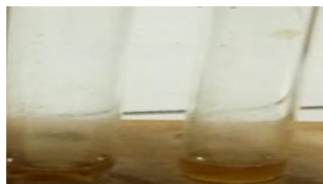
Figure 4. The dark blue or black color did not appear in the tannin test
