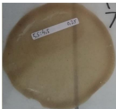
Figure 1. Bioplastics starch: cellulose ratio 5.5:4.5 (g/g) and 0.25 g of filler.
