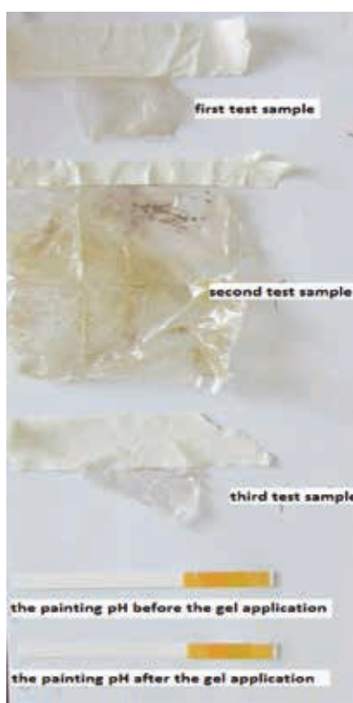
Figure 1. Measuring pH before and after gel application and results for each test.
