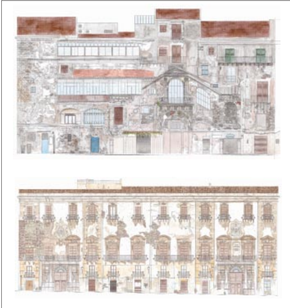
Figures 20-21. Watercoloured iconic representation of the actual state and of macroscopic decays at Vassallo (in front of via Cala), Alliata di Villafranca palaces.
