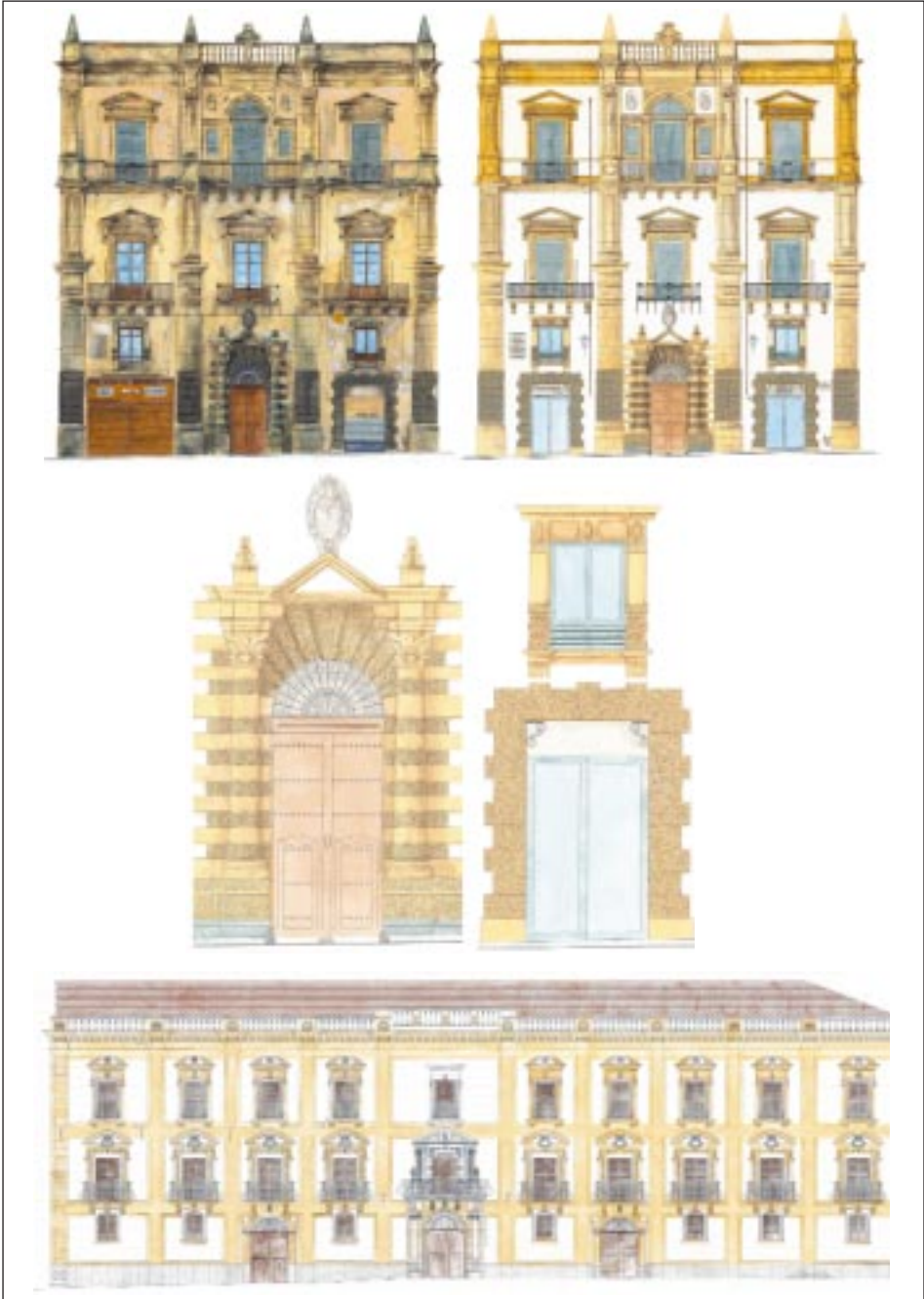
Figures 30-32. Watercoloured iconic representation of reconfiguration hypothesis of Castrone Santa Ninfa, Ugo delle Favare, Alliata di Villafranca, Vassallo Palaces (in front on via Cala), with details of openings on the exterior front.
