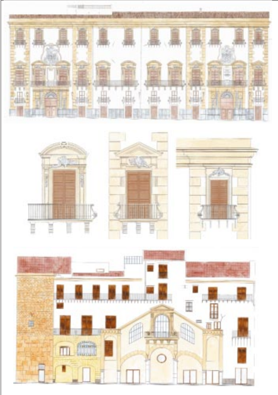
Figures 33-35. Watercoloured iconic representation of reconfiguration hypothesis of Castrone Santa Ninfa, Ugo delle Favare, Alliata di Villafranca, Vassallo Palaces (in front on via Cala), with details of openings on the exterior front.
