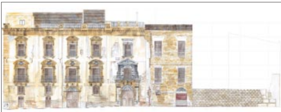
Figure 19. Watercoloured iconic representation of the actual state and of macroscopic decays at Ugo delle Favare Palace.
