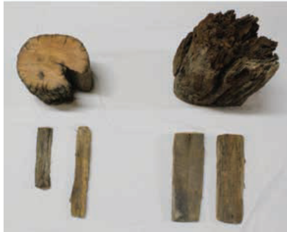
Figure 2. Samples of chestnut wood taken from the beam heads (above) and from the “chiancarelle” boards (below) originally found in structures of the 18 th century (left) and the 19 th century (right).
