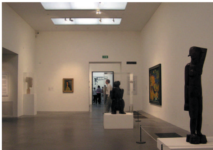
Figure 8. Natural lightening of zenithal type in an exposition room of the Tate Modern of London.
