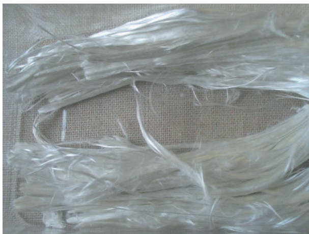
Figure 4. Asbestos fibres contained in an insulating board analysed by microscopy.
