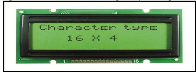
Gambar 3. LCD 16 x 4
