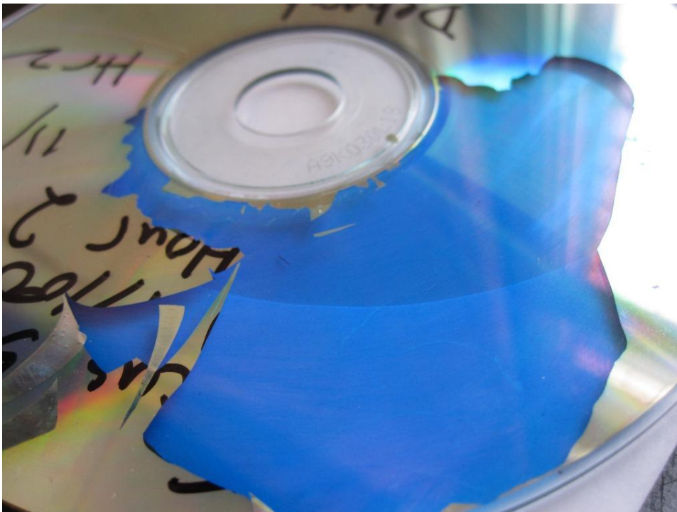
Figure 13. One of several delaminated DVDs located at studios of WILL, Illinois Public Media
