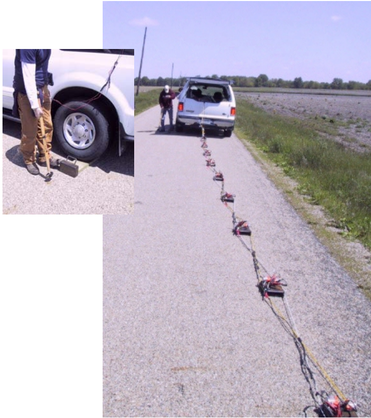
Figure 6. The SH-wave landstreamer in use at Allerton Park. Horizontal geophones are attached to sleds towed behind the car. Inset: the source is a 1-kg hammer striking a plate held under the rear wheel of the car. (from Pugin et al. 2003).
