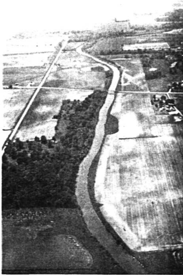
Figure 17. Aerial view of channel of Upper Salt Fork Drainage District, 1974, 80-foot bottom width.
