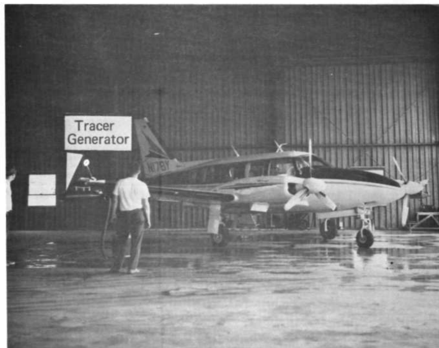
Figure 6. The Atmospherics Inc. Piper Navajo used for the METROMEX project. The tracer release generators can be seen on the wing tips
