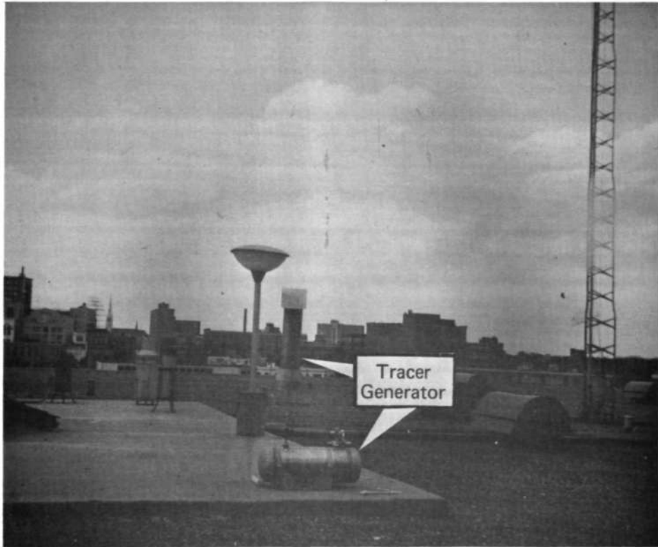
Figure 7. The surface tracer generator provided by the U. S. Navy, Naval Weapons Center for the release of tracer lithium
