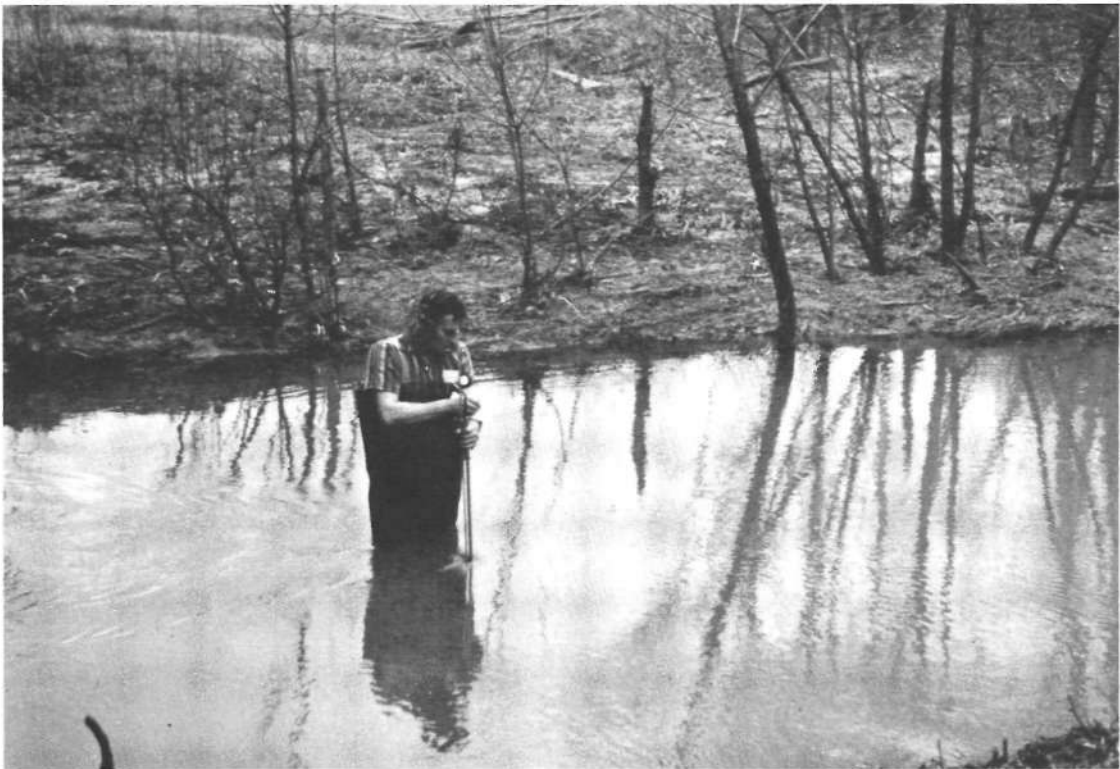
Figure 3. Obtaining a discharge measurement by a current meter and wading, at station 8-0391, Ayish Bayou near San Augustine, Texas, in Neches River Basin
