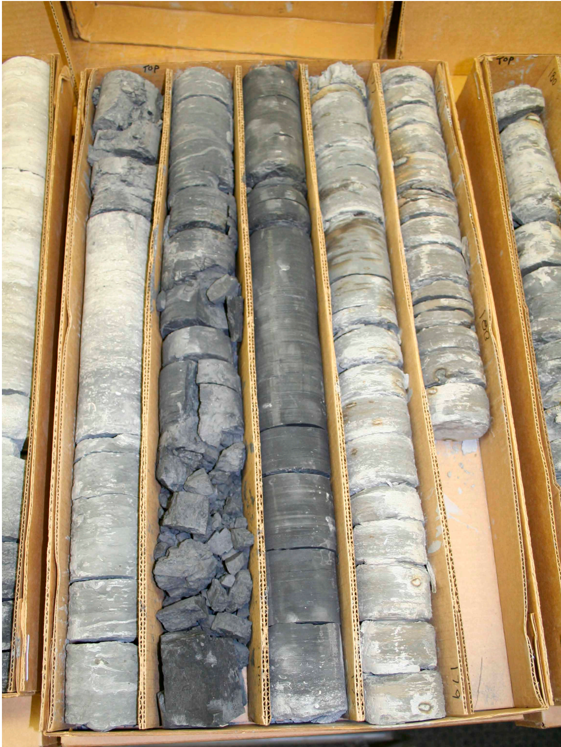
Figure 43 Picture of core from MH-2. The core interval shown here does not encompass either of the depths sampled for x-ray diffraction, but it is representative of the general lithology of the sampled intervals.
