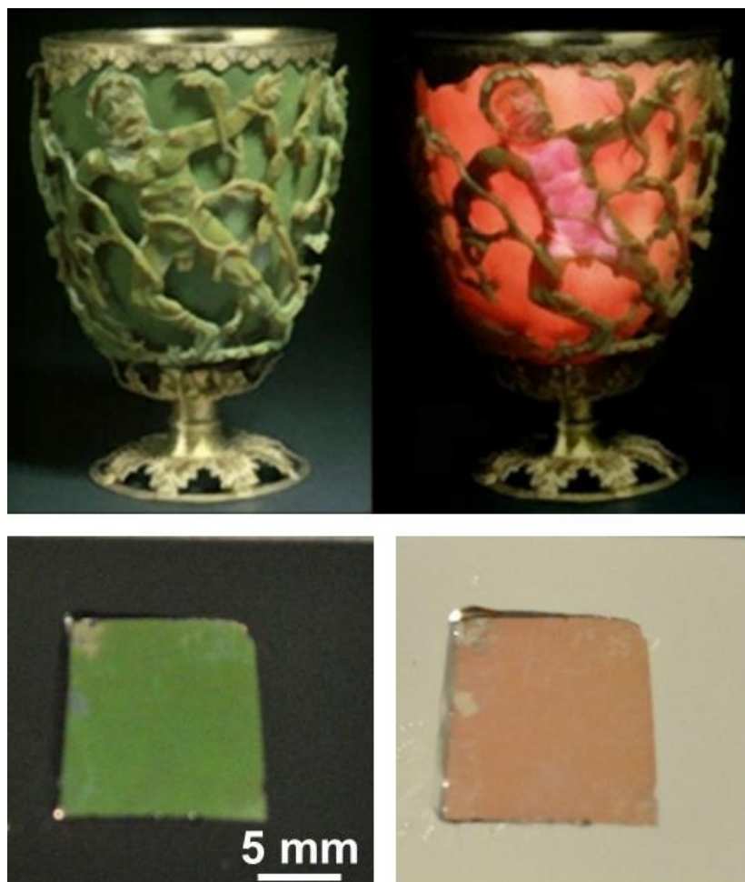
Figure 10.2: The Lycurgus cup in British Museum dated back to fourth century AD. Due to scattering of nanoparticles on sidewall (5-60 nm in diameter), the cup appears green in reflected light and appears red in transmission light. Optical micrograph of nanoLCA taken using a camera under direct illumination (green) and without illumination (red) of Xenon lamp flashlight.
