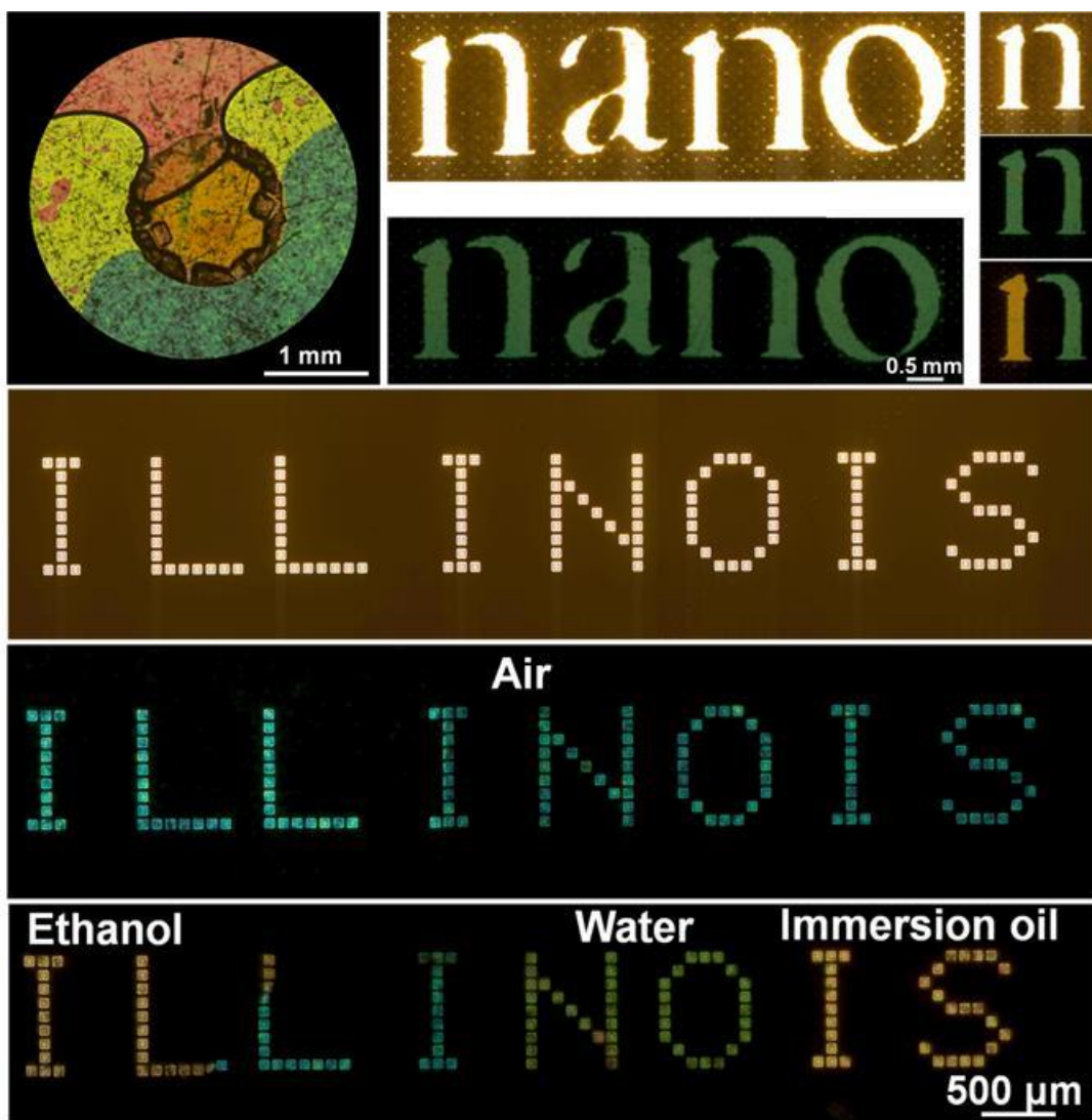
Figure 10.13: Creation of vibrant colors in transmission mode image of nanoLCA with mixture of NaCl, immersion oil and ethanol. The word ‘NANO’ was printed on a transparency sheet and nanoLCA device was kept on top of it. Light was illuminated from the bottom of the transparency. An ethanol drop was placed on part of the letter ‘N’ which appears orange in the transmission image. The rest of the letter is green due to the transmission property of nanoLCA. To illustrate the high spatial control, a lithography mask in quartz with the word ‘ILLINOIS’ was made and light was transmitted from the bottom of the mask while the nanoLCA sitting on top of it. The color appears green with air interface but changes to orange, light green and red for ethanol, water and immersion oil interfaces respectively.
