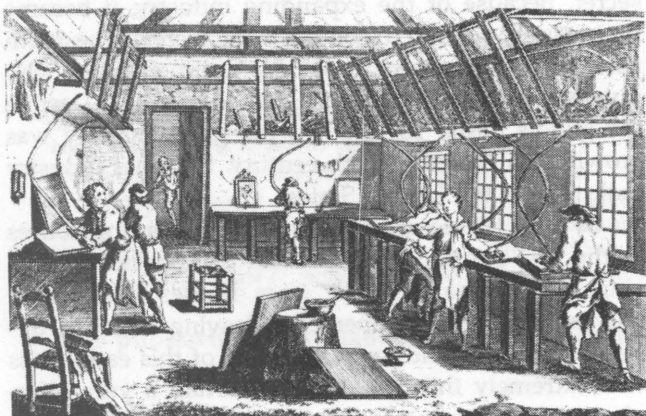
Inside a glass factory in the 1700's, plate glass was ground and polished by hand.
